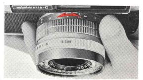
To focus, center the small rectangle over the center of interest in the scene and rotate the Distance Control Ring until the two images merge, forming one clear image. The camera is now in focus for this particular picture.
