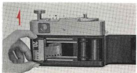
Pull out the Film Rewinding Knob, and insert a new roll of 35mm film in the film chamber.
