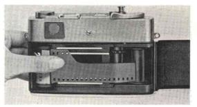
Thread the film leader into the slot of the Take-up Spool in the film chamber.
