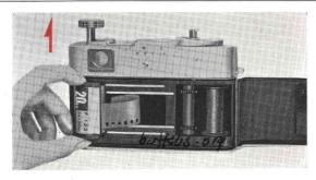
When the film is completely rewound into the casette, open the back cover by pressing the Back Cover Release Button in the direction of arrow and down. Pull up the rewind crank shaft and remove casette.
