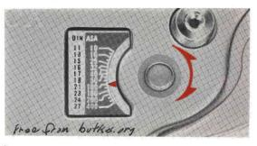
To set the proper film speed (ASA or DIN), pull up ASA (DIN) Film speed setting Knob and turn it until the needle is opposite the index number of the film to be used. This number is found in the film instruction sheet.
