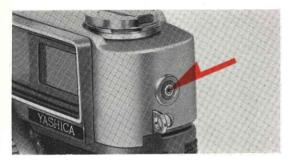
Insert the electronic flash unit's sychro-cord into the "X" flash terminal on the side of the camera, body. Now that an "X" synchro-terminal and 1/30 second shutter speed are provided, use electronic and either "F" or "M" class flash bulbs.
