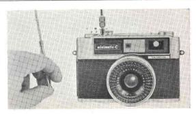
When using "B" setting, remember that a cable release and tripod are to be used. The Cable Release can be screwed into the socket provided in the Shutter Release Button.
