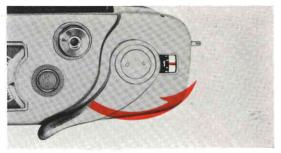
■After the back cover locks into position the Film Exposure Counter will be automatically set to "S" (start), then advance the film and press the Shutter Release Button. Repeat the same operation until the figure "1" appears in the Exposure Counter Window. Take Your first picture.
