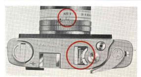
To set the proper film speed (ASA or DIN), pull up ASA (DIN) Film Speed Setting Knob and turn it until the needle is opposite the index number of the film to be used. Turn the Lens Opening Control Ring counterclockwise until "AUTO" is opposite the red indicator line.
