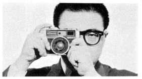
It is very important to hold your camera correctly and steadily when taking pictures in order to obtain good results. Hold it close to your face with your elbows held close to your waist, so that blurring will not occur. The picture at the left shows how to hold your camera in the horizontal position.
