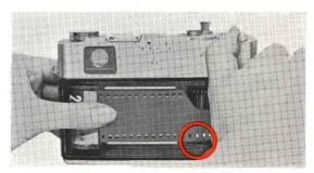
Madvance the film with one stroke of the Advance Lever, and make sure the perforations of the film fit over the sprocket teeth.
