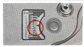
Proper exposure of these scenes may be obtained, automatically, by simply resetting the ASA (DIN) Film Speed Setting Knob to half of the speed of the film in use. Remember to reset ASA speed index for normal scenes after use.
