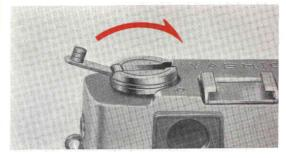
Flip up the film rewind crank to the horizontal position and turn in the direction of arrow. Toward the end of the film you will feel a slight resistance. But continue turning the rewind crank until the film pulls away from the slot on the Take-up Spool.
