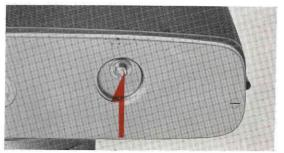
Press the Film Release Button which is located on the base of the camera. The Film Release Button need not be kept depressed while the film is being rewound.
